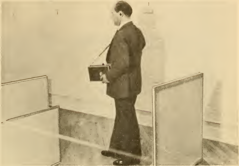
FIG. 3.5 SUBJECT CARRYING BRUSH SUPERSONIC GUIDANCE DEVICE, YA-3 BD.
