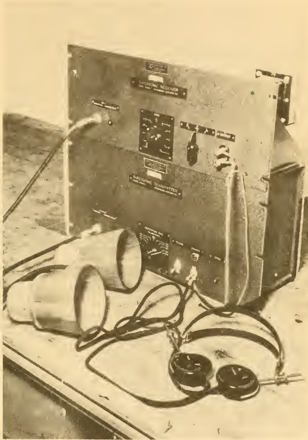
FIG. 2.7 NON-PORTABLE MODEL OF STROMBERG- CARLSON'S TWO-CLICK SYSTEM, YA-1ST.
