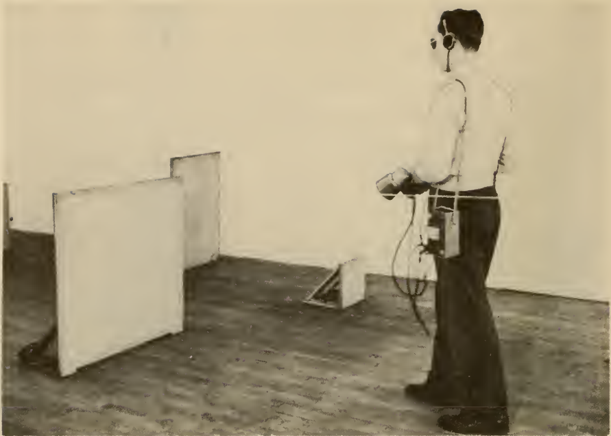
FIG. 3.3 SUBJECT CARRYING STROMBERG-CARLSON "PULSED FM" SUPERSONIC GUIDANCE DEVICE, YA-3 ST.
