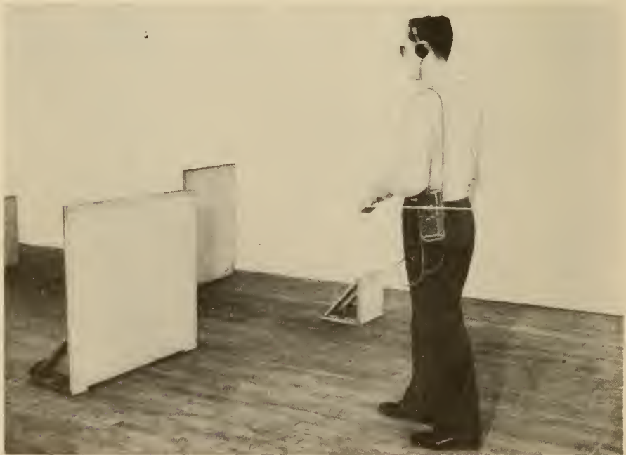
FIG. 3.4 SUBJECT CARRYING BRUSH SUPERSONIC GUIDANCE DEVICE, YA-5 BD.
