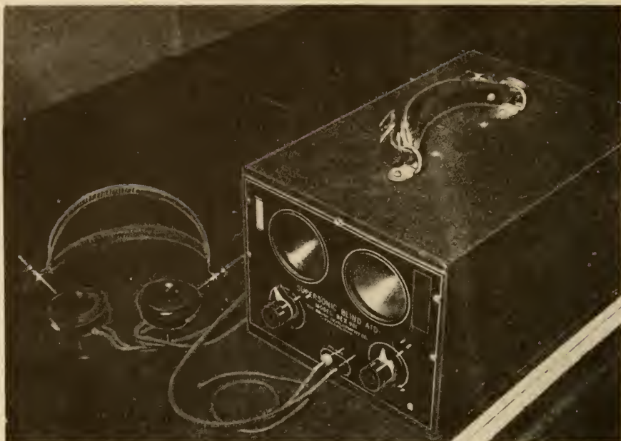
FIG. 2.20 BRUSH SUPERSONIC SINE-WAVE MODULATED GUIDANCE DEVICE, YA-IBD.
