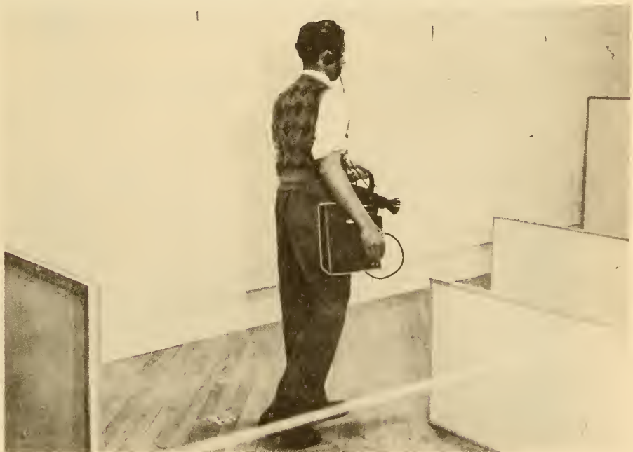
FIG. 3.6 SUBJECT CARRYING HOOVER MECHANICAL SUPERSONIC GUIDANCE DEVICE, YA-1 HC.
