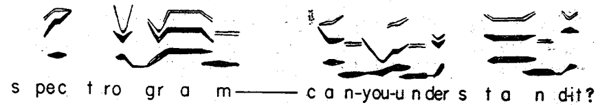
FIGURE 3 An Early Example of a Reduced Spectrogram Painted by Rule for Use with the Pattern Playback
