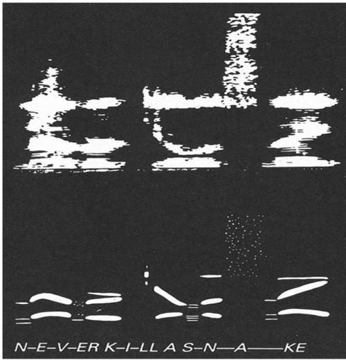
Figure 4. Negative of a spectrogram of the sentence fragment *Never kill a snake* (top) and a schematic copy for input to the Pattern Playback (bottom).
